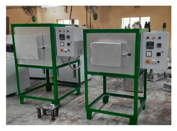
Our Muffle Furnaces are excellent in performance over a long period of time & are suitable for a wide range of applications. Muffle furnaces give trouble free performance at substantially high temperature i.e. 1000 – 1200C. We present a wide range of muffle furnaces mainly built for laboratories and production industries. These muffle furnace models are durable from top to bottom, energy efficient and perfectly work in all conditions.
